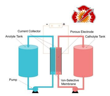
The chosen electrolyte is based on the system design. This paper will address only Vanadium Redox as it is currently considered one of the safest flow battery technologies currently available. This is supported by operational and test data available from 20+ years of systems installed in various different applications, environmental conditions, and product configurations world-wide.
